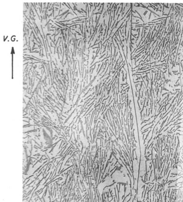
Figure 14 The irregular structure of Al-Si eutectic during directional solidification. V = 10.0 \mu\text{m s}^{-1} , G = 89 \text{K cm}^{-1} , longitudinal section.
